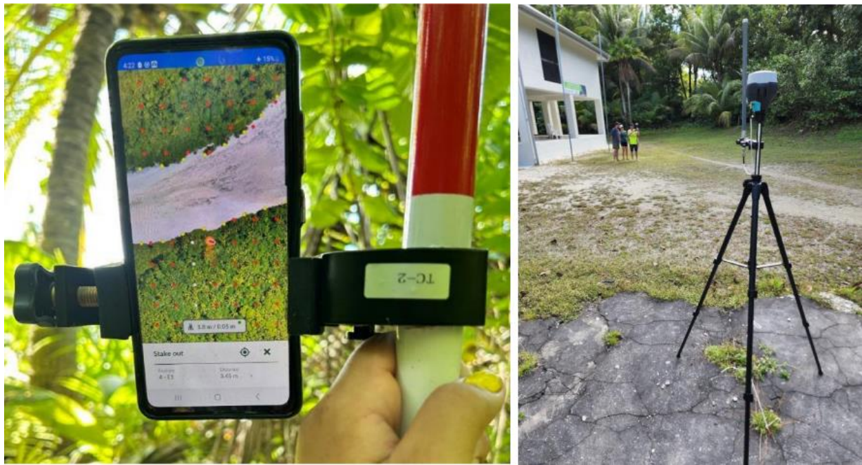
Figure 7 – Mergin maps mobile data collection and navigation project being used with an RTK rover pole to establish a baiting grid on Palmerston Atoll, Cook Islands (left). An Emlid RTK unit set-up as a base RTK unit on Palmerston Atoll, Cook Islands. Images and information courtesy of Department of Conservation, New Zealand.
