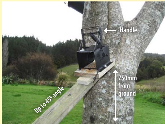
FIGURE 13A. To mount the trap, place it on a wooden ramp at approximately 750mm above ground level, on an angle of up to 45 degrees, against a sturdy tree or structure. Screw the trap into position (an 8mm socket on the end of a battery drill works well).
