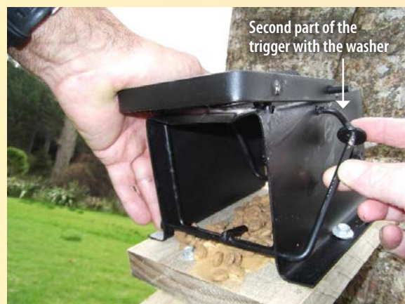
FIGURE 13D. While holding down the handle, rotate the front part of the trigger up into the second half of the trigger with the washer. The parts should fit together in the set position. Fingers must not be anywhere near the inside of the trap! The final act of luring the trap is to throw in a handful of cat biscuits. You can place additional lures outside the trap to entice the cat into it.
