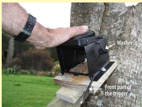
FIGURE 13C. To set the trap, stand in front of the secured trap, with the front part of the trigger pointing at you. It is important to use the correct hand orientation to set the trap - a flat palm with fingers pointing to rear of the trap. Pull then push down the handle, using a reasonable amount of force.
