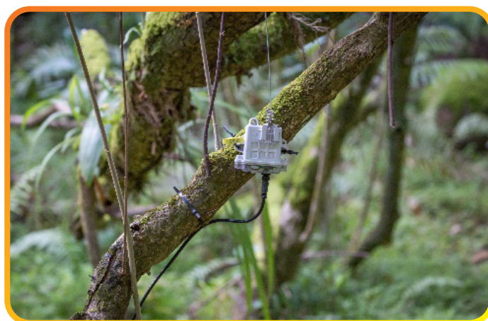
FIGURE 9. Node for satellite network of cat traps on Fatu Hiva. Photo: B. Ignace
