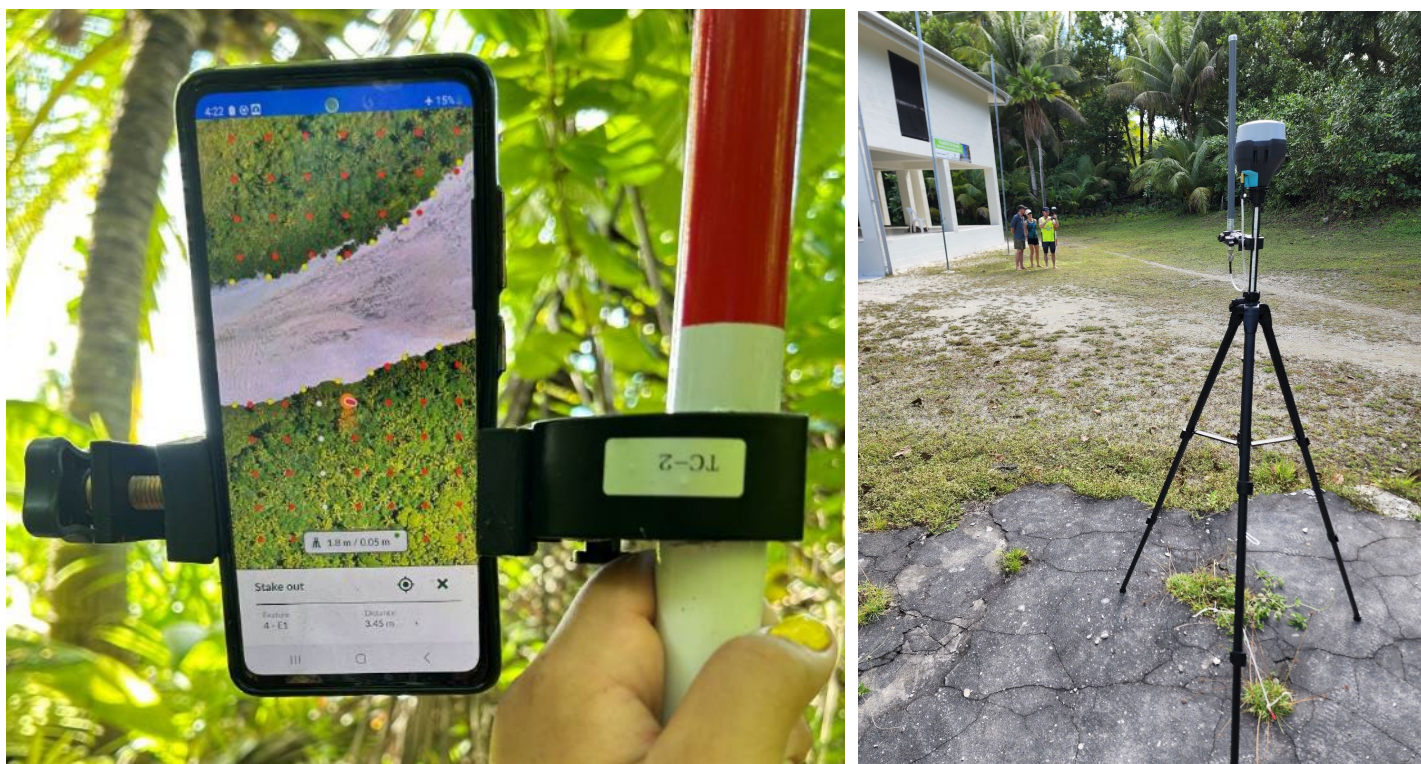
Figure 2.7: Mergin maps mobile data collection and navigation project being used with an RTK rover pole to establish the baiting grid (left); an Emlid RTK unit set up as the base RTK unit on Home Island (right)
