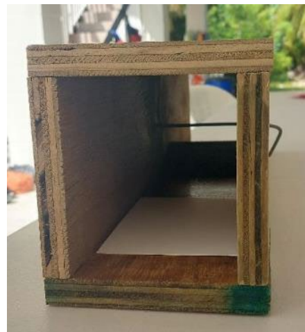
Appendix 4.2.4: Wooden tunnel with tracking card installed. Wire peg can be used to hold bait (toasted coconut flesh)
