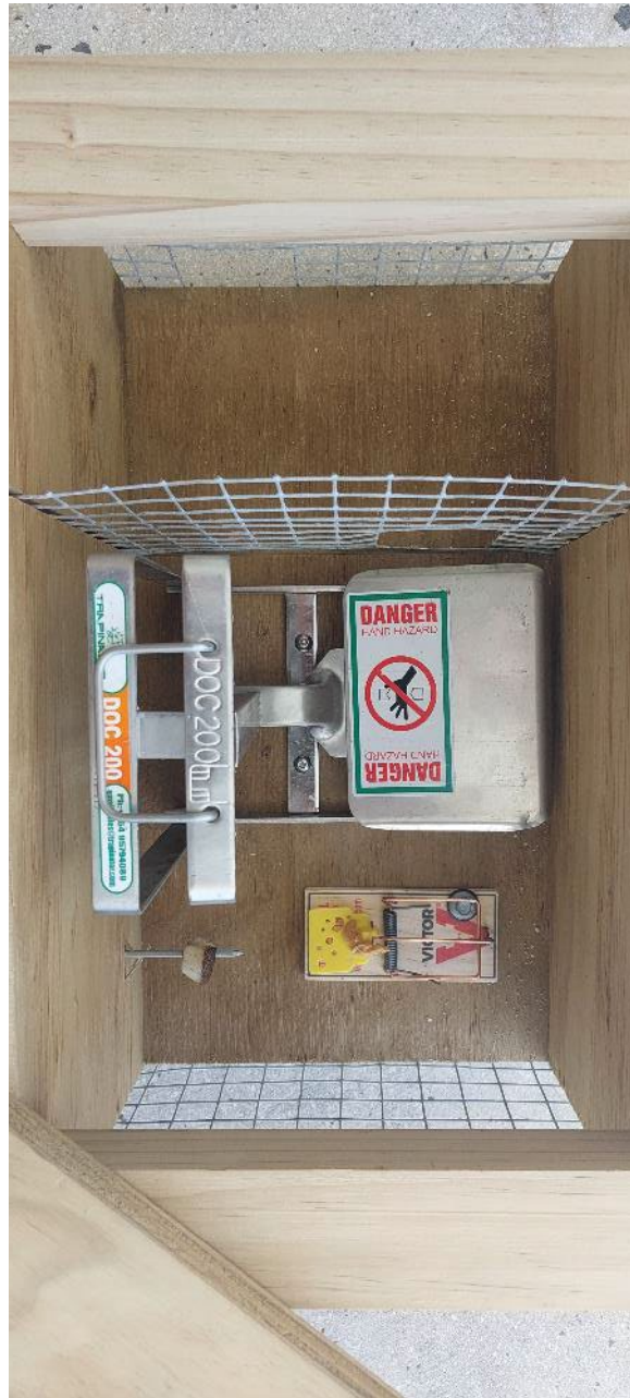
Appendix 4.2.5: DOC200 trap box with mouse trap. Traps set and ready, with toasted coconut flesh on side bait nail, and mouse trap baited with peanut butter.
