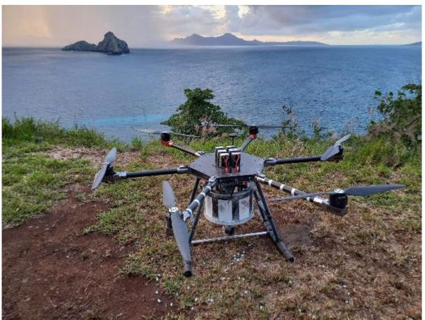
Figure 10 - a battery operated drone with bait spreader bucket attached at the loading site during a Pacific rat (Rattus exulans) eradication on Kamaka, French Polynesia.
