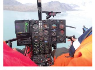
Fig. 4 TracMap<sup>™</sup> GPS guidance equipment fitted to South Georgia Heritage Trust aircraft,2015.
